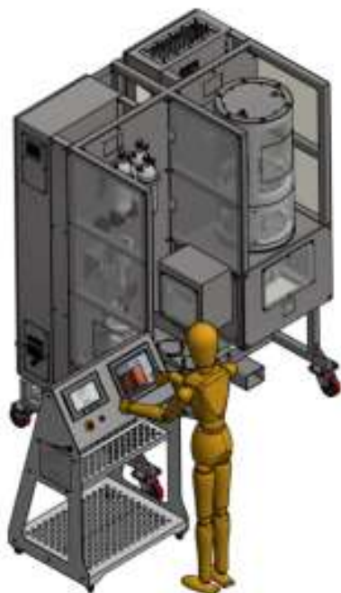
Representative Arrangement of a CCFD50 Vision Filter Dryer
