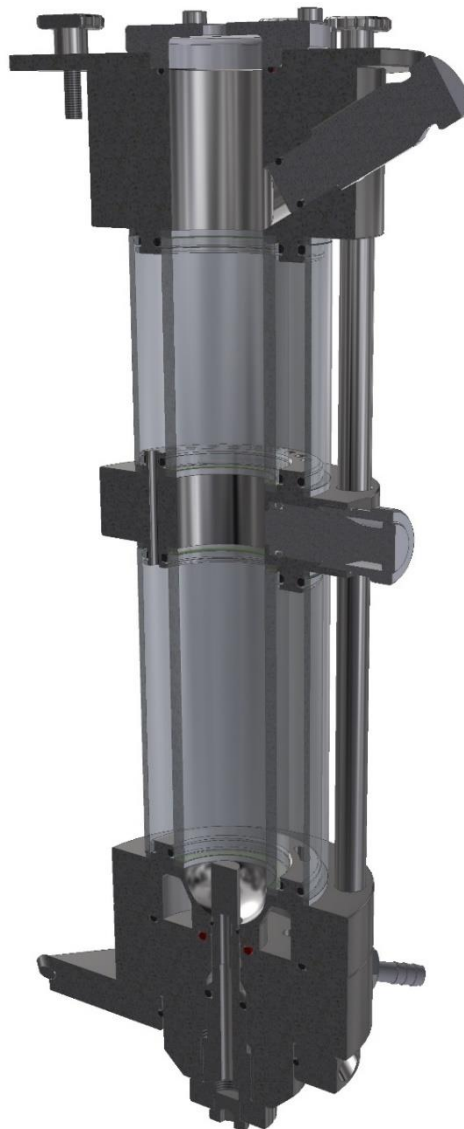
Figure 1: Cross section view through a reaction vessel
